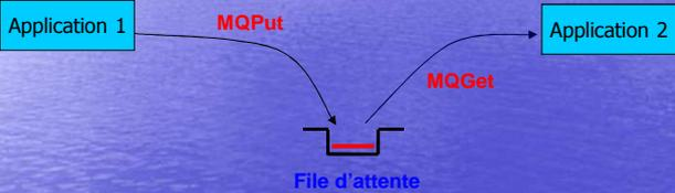
The diagram illustrates a traditional messaging flow. On the left, a box labeled 'Application 1' has an arrow pointing to a central 'File d'attente' (queue) icon. This arrow is labeled 'MQPut'. From the 'File d'attente' icon, an arrow points to a box on the right labeled 'Application 2', which is labeled 'MQGet'.
